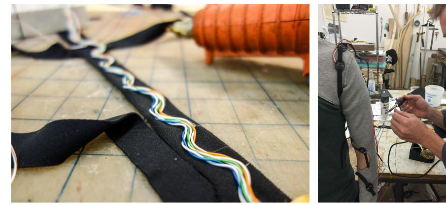
Our final prototype was built into a short jacket and used sliding buckles to adjust to the user. It was powered by an x-OSC board.
