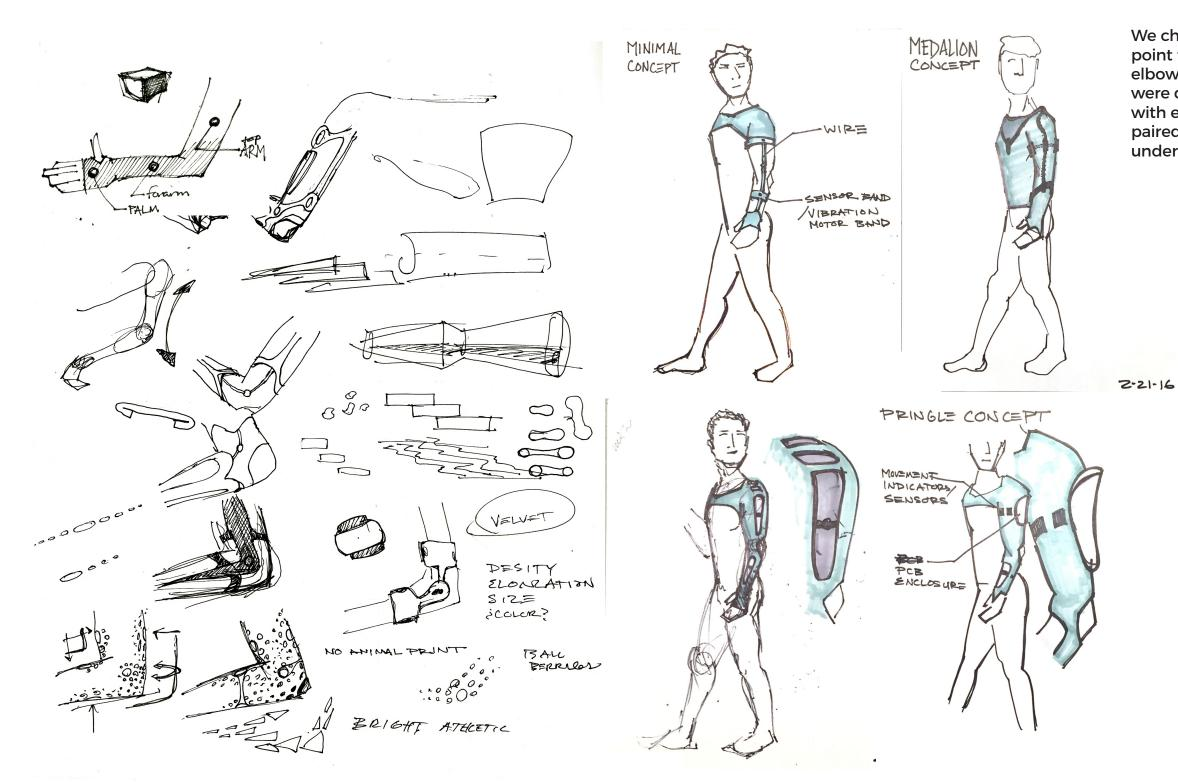
We chose the arm as a starting point for the binary nature of the elbow joint. Various concepts were developed for a short jacket with embedded electronics paired with a long sleeve shirt underneath.
